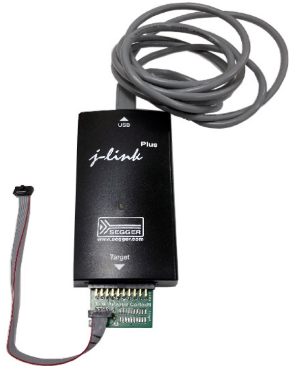
Figure 3: Segger J-Link PLUS for SWD Configuration (Baseboard and I/O Expansion)
